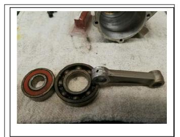
The connecting rod and both bearings needed to be replaced.
