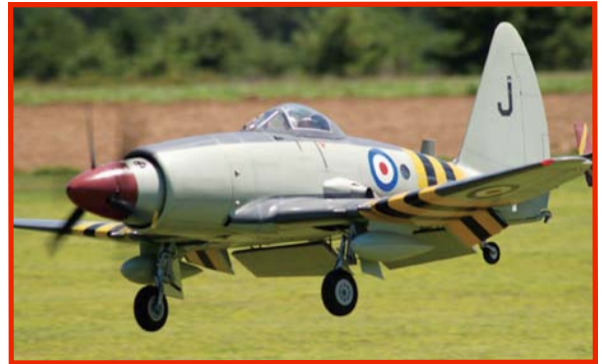
This impressive Westland Wyvern is the work of David Wigley. The model weighs 50 pounds and features scale Fowler flaps, which increase both drag and wing area when deployed.
