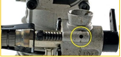
With a single-needle carb, there is a small air-bleed hole in the front for the low-end idle mixture. You adjust the mixture screw to open and close the hole to adjust
