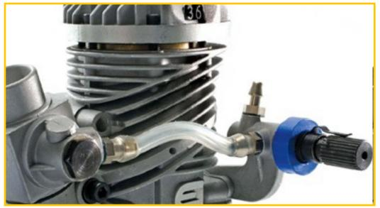
Many newer engines such as this Evolution .36 2-stroke, have their high-end needle valve assemblies placed in the rear of their engines away from the prop. It is connected to the carb with a short piece of fuel line.
