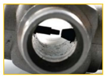
As the throttle barrel closes, the low-end needle assembly moves laterally into the fixed spray bar. This is why adjusting the low-end needle affects the high-end mixture adjustment.
