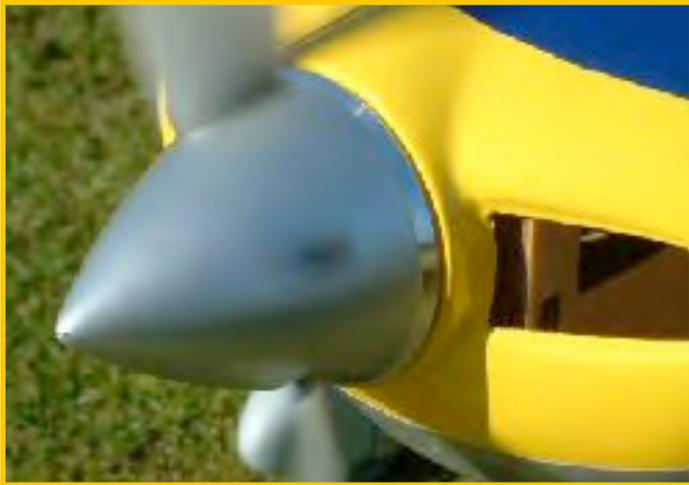
Trying out a few different propellers can produce a surprising performance gain. Remember to balance the spinner as well.
