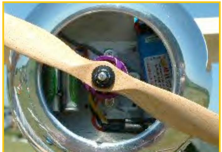
A balanced propeller will not waste motor power producing vibration - instead, all of the motor's output power will go into turning the prop.
