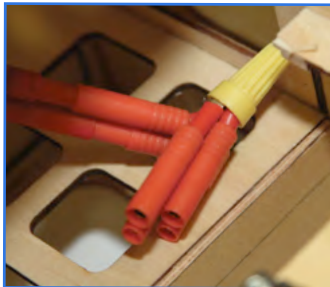
A homemade parallel battery connector in a plane; wire nuts belong at home, not in your plane..
