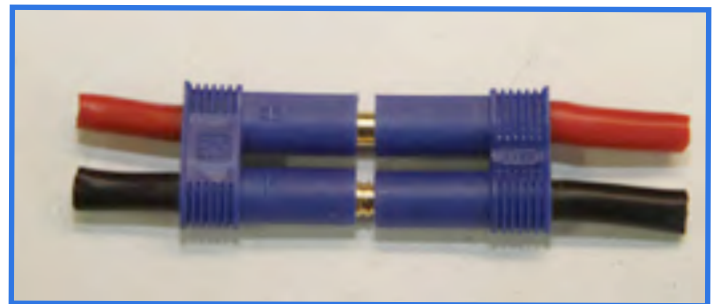
An improper extension made by jamming a bullet into the EC5 connectors. Great
