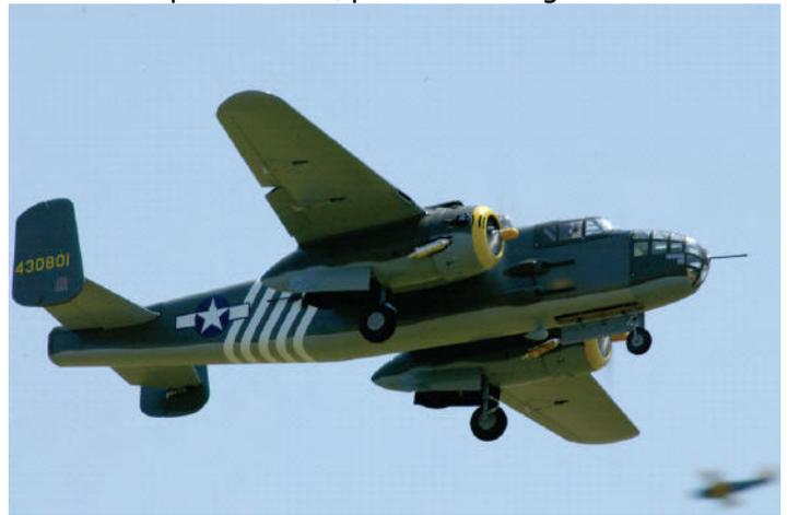
The Top Flite B-25 Mitchell bomber has inboard and outboard flaps because of its twin wing-mounted engine nacelles. With the flaps deployed, this impressive warbird ARF lands like a trainer.
