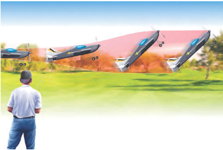
Figure 1: During a Harrier, the plane slowly flies across the field at a high angle of attack
