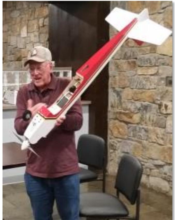
He even replicated the radio setup that he was using at that time. While the radio still is using 72 MHz he has upgraded to a Futaba RF module with Futaba servos. The plane is covered in SolarTex for that authentic look and has an Enya 45 for power. Vintage to the
